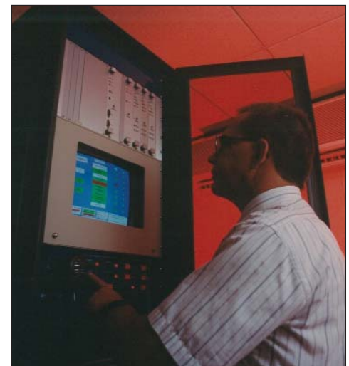
Touch screen monitor is a user-friendly way to supervise RF links and remote station status.
